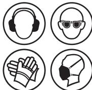
Personal Protective Equipment (P.P.E.), such as ear defenders, eye protection, safety gloves and a dust mask, must be worn during the operation of the device.
